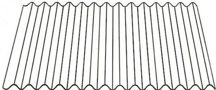
**N**u-Wave® Corrugated is a through-fastened metal panel with 7/8" deep corrugations. The panel measures 36" out-to-out, with a 32" net coverage for roof applications and a 34 2/3" net coverage for wall application
