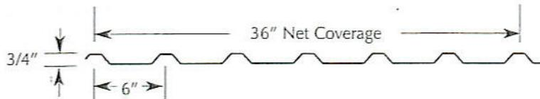
**U**-Panel is a "Utility" panel known for its economical through-fastened design preferred for light commercial and industrial roof or wall applications. U-Panel is especially suitable as an interior partition or liner panel for mini-storages.
