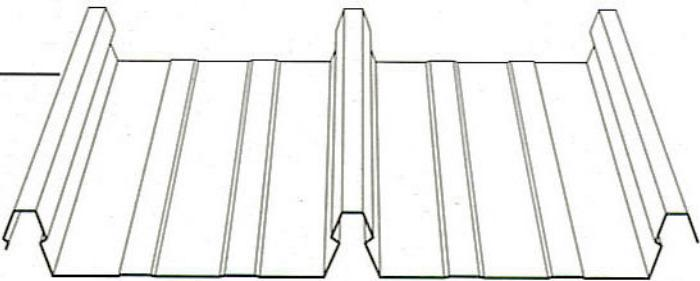
**K**lip-Rib® is a performance rated structural and architectural standing seam panel system that snaps positively over concealed anchor clips for quick installation and exceptional strength. Klip-Rib® is the preferred panel for commercial, educational and institutional roofs in all climates.
