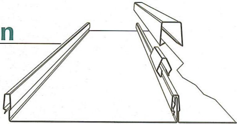
Design Span® Batten is a high performance structural standing seam metal roof system with net coverage of 12" up to 24". Design Span is excellent as a roof over metal or wood decking, and as a fascia or mansard over plywood or supports.
