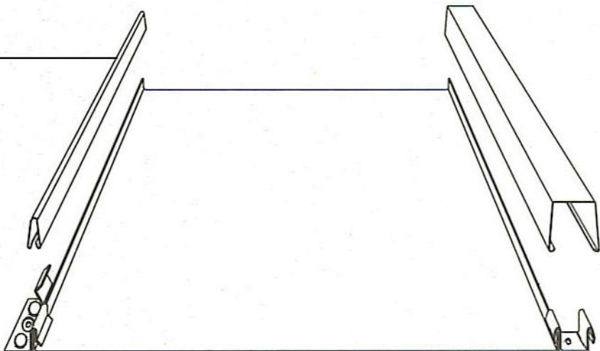
**S**elect Seam is a performance-rated, non-structural, batten seam metal roof system. It's clean wide pan appearance makes it ideal for a classic architectural effect.
